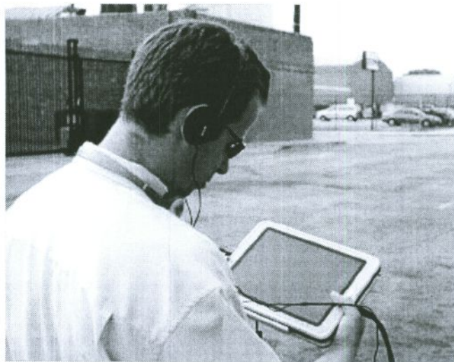
Photograph 1. The system includes a tablet computer with a built-in GPS receiver and audio headphones.
